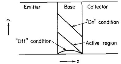
FIG. 16-2. Minority-carrier concentrations in the base layer as related to the region of operation.
