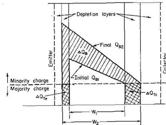
FIG. 16-5. Base-charge distributions illustrating switching in the active region. The shaded area denotes additional stored charge.
