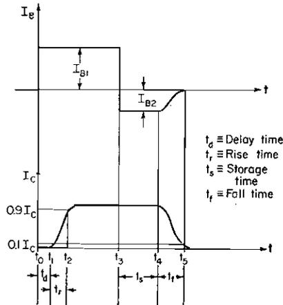
FIG. 16-4. Input base-current waveform and output collector-current waveform for a transistor, illustrating definition of switching times.
